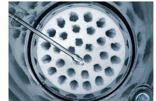
Single shake back filter system.
